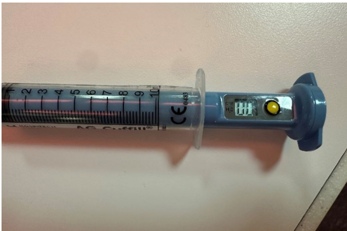
Figure 4. Digital manometer may be used for more precise measurements.
